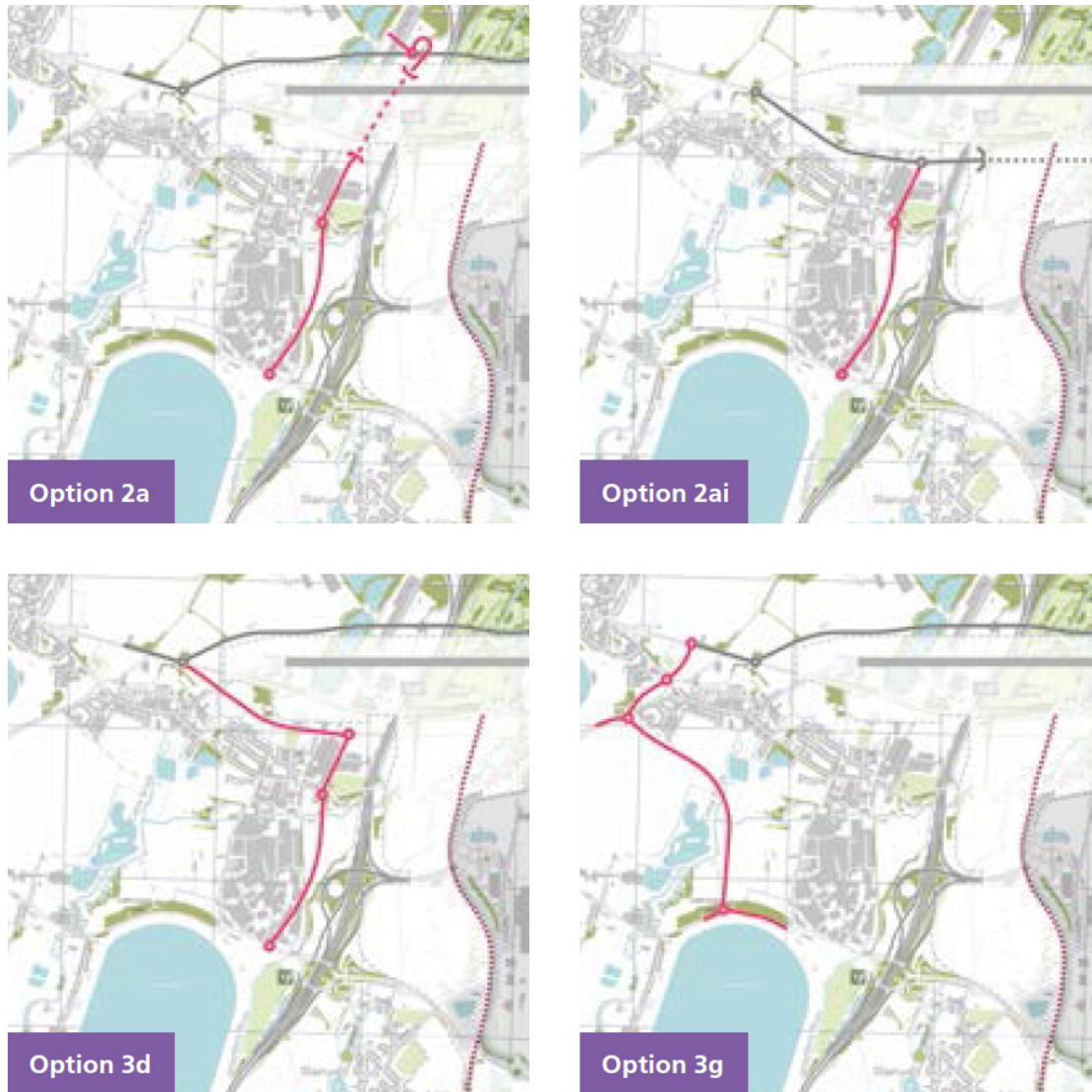
Figure 1: Options for the relocation of the A 3044 through Colnbrook & Poyle
